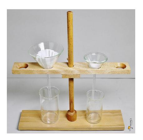
A filter rack is a used for funnels during filtration. They make sure that the funnels are always positioned vertically.
