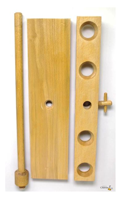
As the assembled filter rack takes up a lot of space, it is typically found in its components in the lab.
